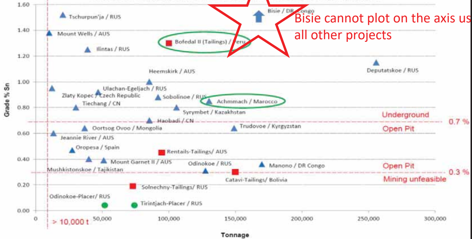
Comparison of tin deposits which can be mined feasibly at current tin prices
